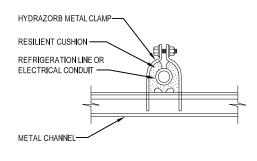
NOTE: ALSO APPLIES TO INSULATED SUCTION LINES AT THE FIRST THREE SUSPENSION POINTS FROM THE COMPRESSOR.
